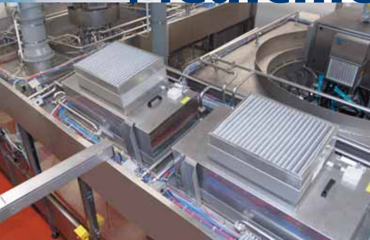
Supply and exhaust air system on an aseptic filling machine in the beverage industry
