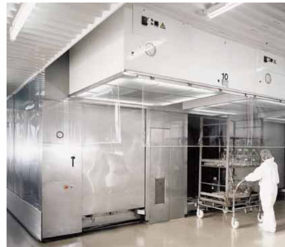
Hot air sterilization, low-maintenance outlay and no risk from cross-contamination
