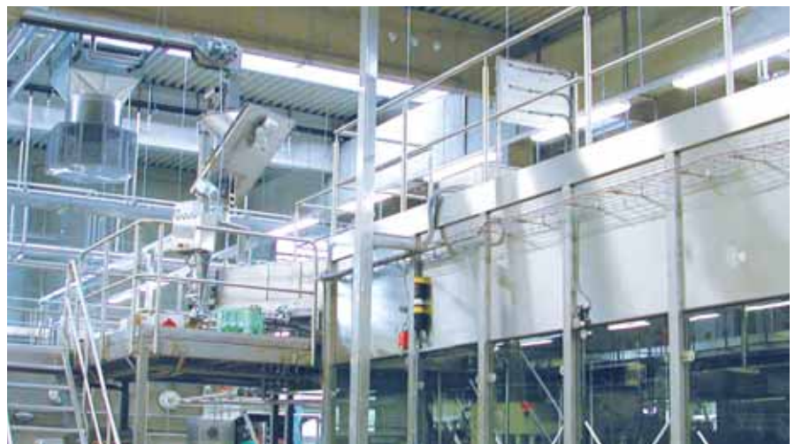
ULTRACLEAN® clean room housing for filling machinery in production facilities
